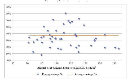
Note: Energy savings are here expressed in % of the energy consumption before renovation (including space heating and domestic hot water). The average energy savings is about 37%, with a spread from 9% to more than 70%. Considering space heating only, the average savings are about 32%.
